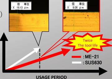
\*Test result of Company A (positive electrode) Hardness of paste: Hv1000 Due to NDA, unable to give other details
