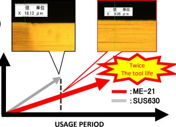
\*\*Test result of Company A (positive electrode) Hardness of paste: Hv1000 Due to NDA, unable to give other details
