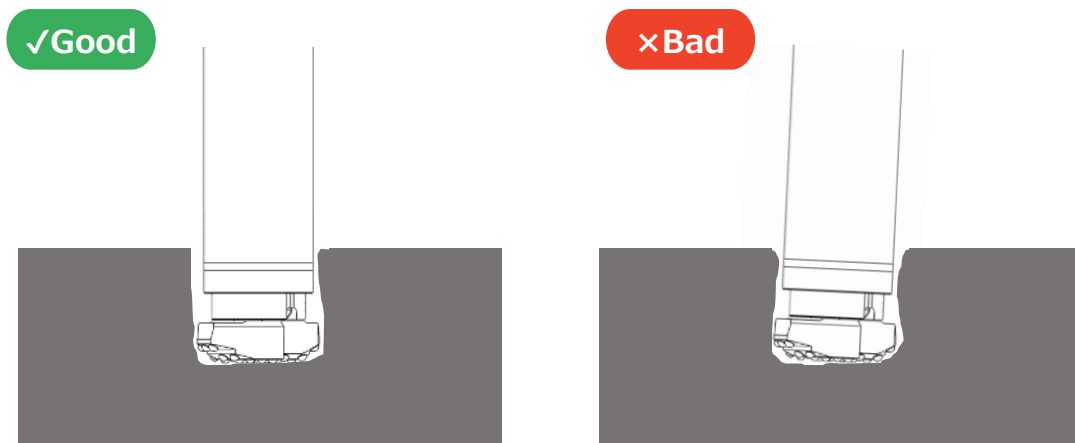
Figure7: Checking the casing pipe alignment
